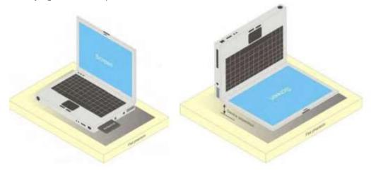
Test positions for Body-supported Device
