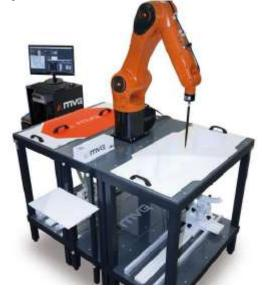
The EUT under test operating at the maximum power level is placed in the phone holder, under the phantom, which is filled with head simulating liquid. The E-Field probe measures the electric field inside the phantom. The OpenSAR software computes the results to give a SAR value in a 1g or 10g mass.
