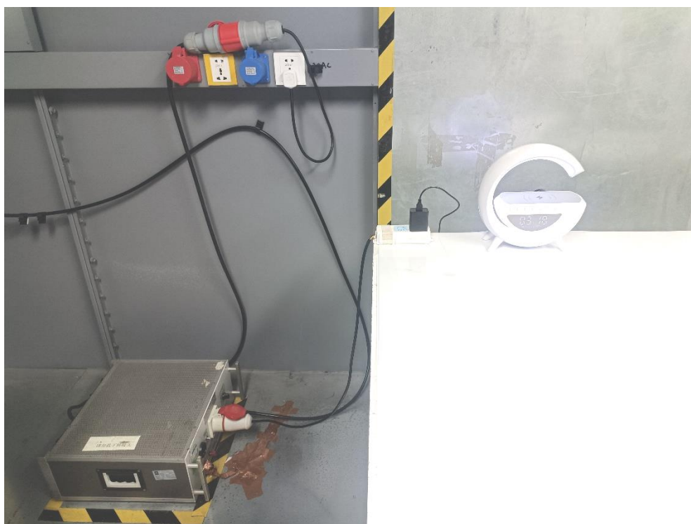
Photo of Conducted Emission test
