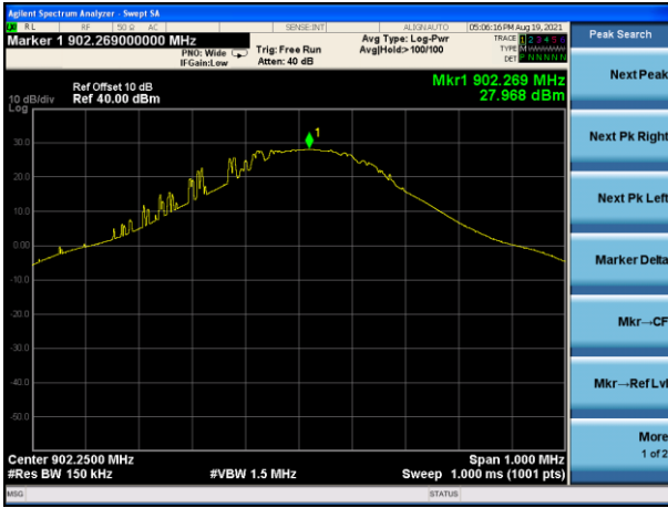
Peak output Power plot on channel 25 (1Mbps)
