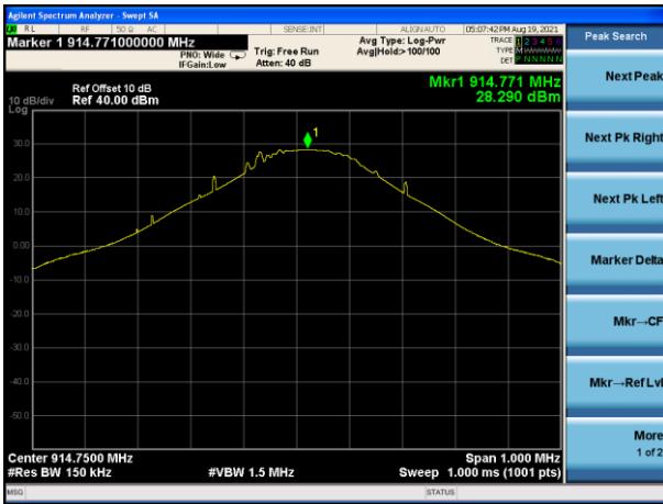
Peak output Power plot on channel 51(1Mbps)
