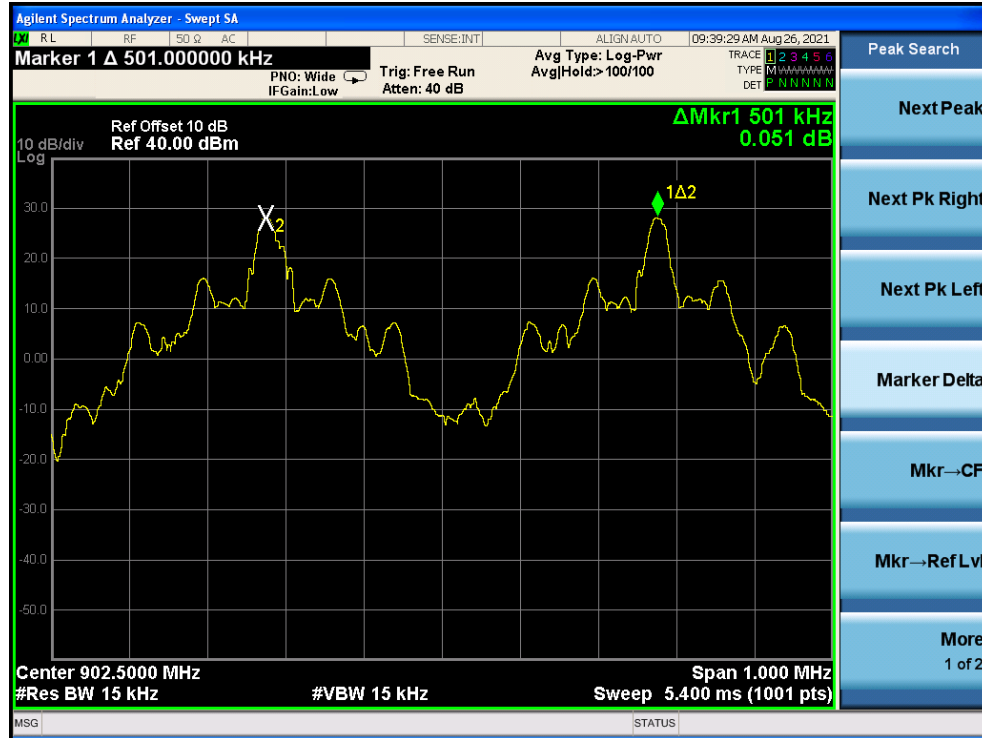
(1Mbps) Channel Separation plot on channel 00-01
