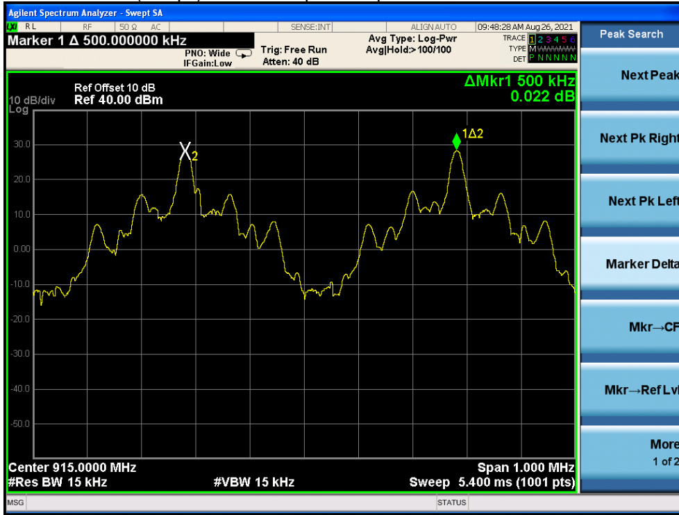
(1Mbps) Channel Separation plot on channel 50-51
