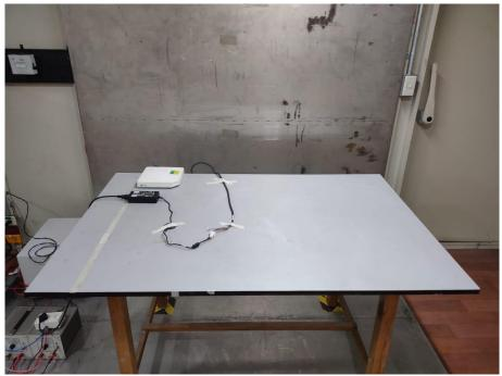
1.3 Radiated Emission Test Setup
