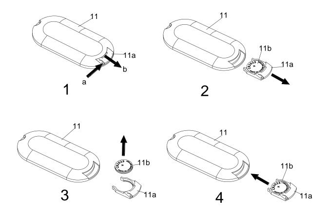
Press the arrow to squeeze point A of battery seat (NO.11A), and buckle point B of battery seat (NO.11A), and pull out b attery seat (NO.11A). Take out the old battery (NO.11B), put the new battery into the battery seat (NO.11A), and finally insert it into the Romote Control (NO.11).
