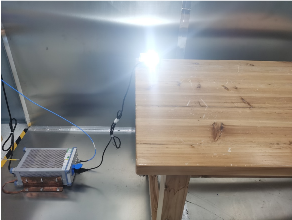
Photograph 3: Set-up for Conducted Emissions ON AC mains
