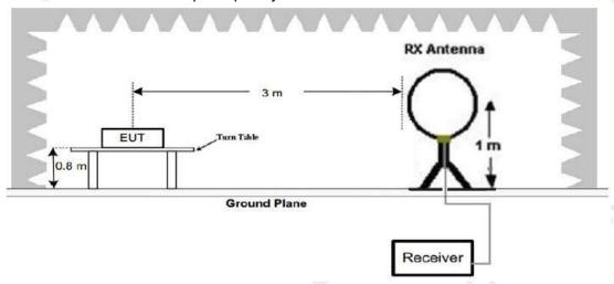
2. Radiated Emission Test-Up Frequency 30MHz~1GHz
