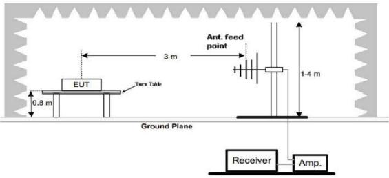
3. Radiated Emission Test-Up Frequency Above 1GHz
