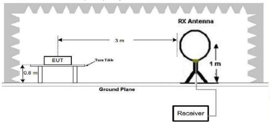
2. Radiated Emission Test-Up Frequency 30MHz~1GHz
