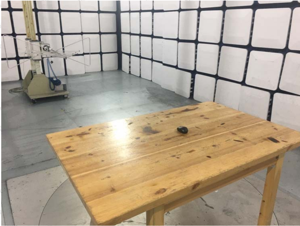
Photo of Radiation Emission Test
