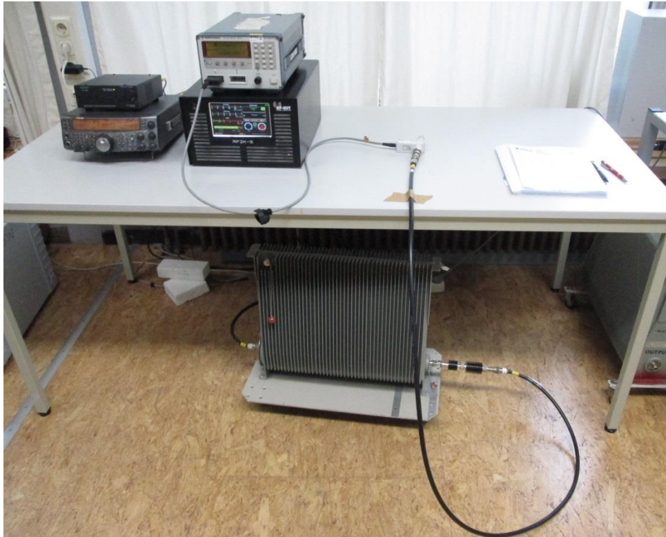
Photo A1-1: Conducted amplifier gain emissions measurement
