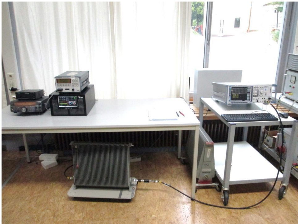
Photo A1-2: Conducted amplifier spurious emissions measurement
