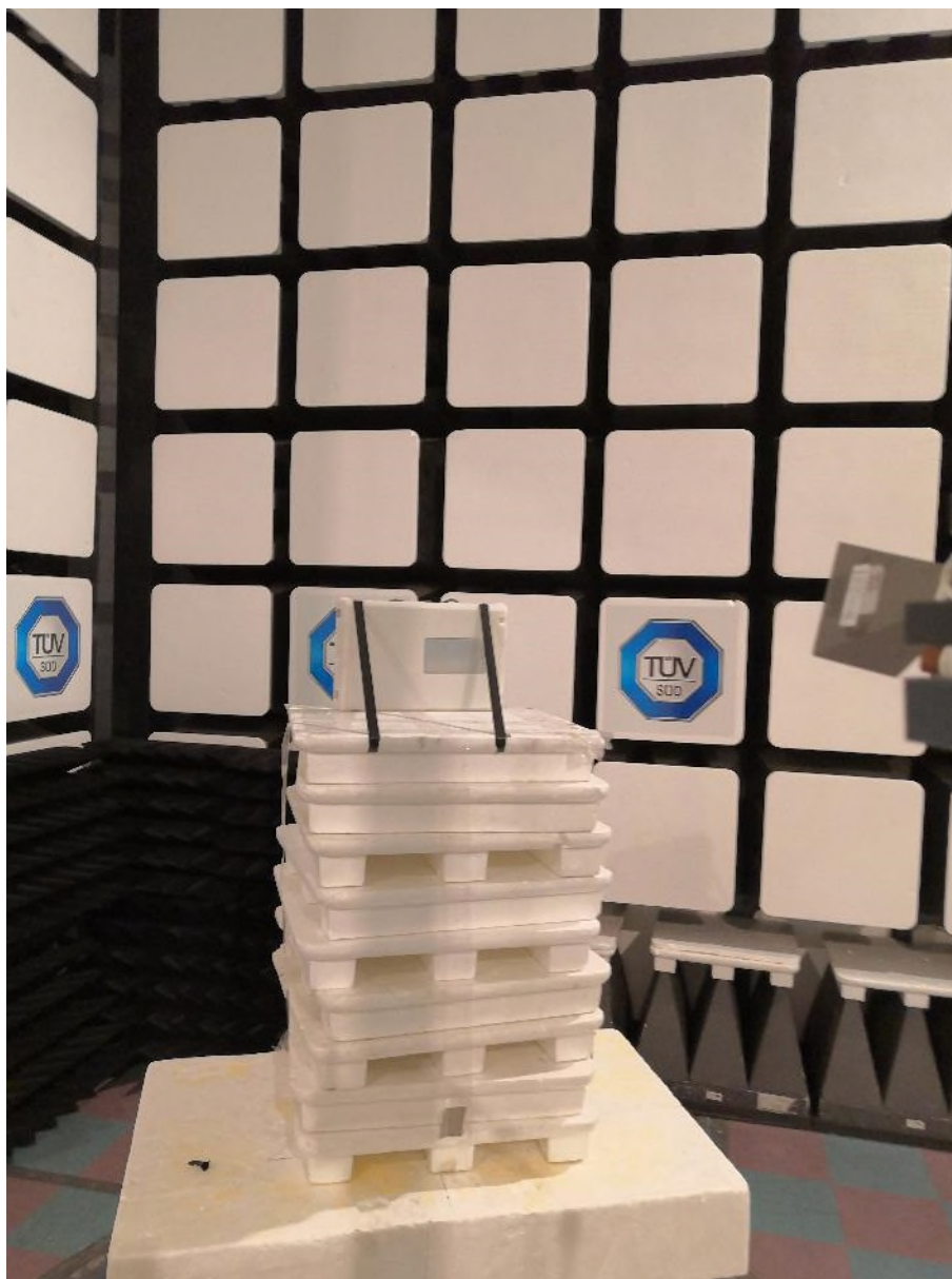
Figure 5 – Radiated Emissions Setup 18GHz to 26GHz Spurious Scans
