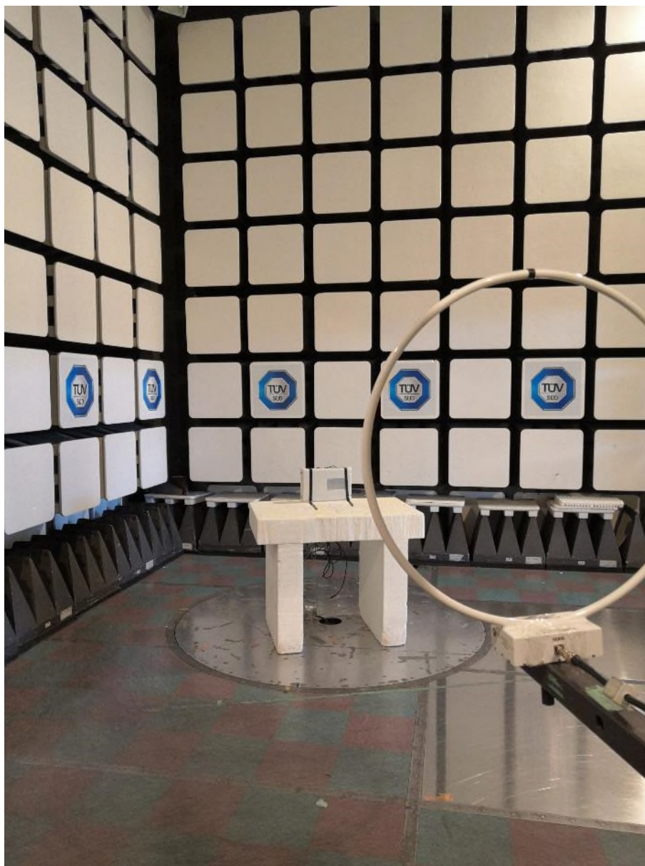
Figure 1 – Radiated Emissions Setup 9kHz to 30MHz
