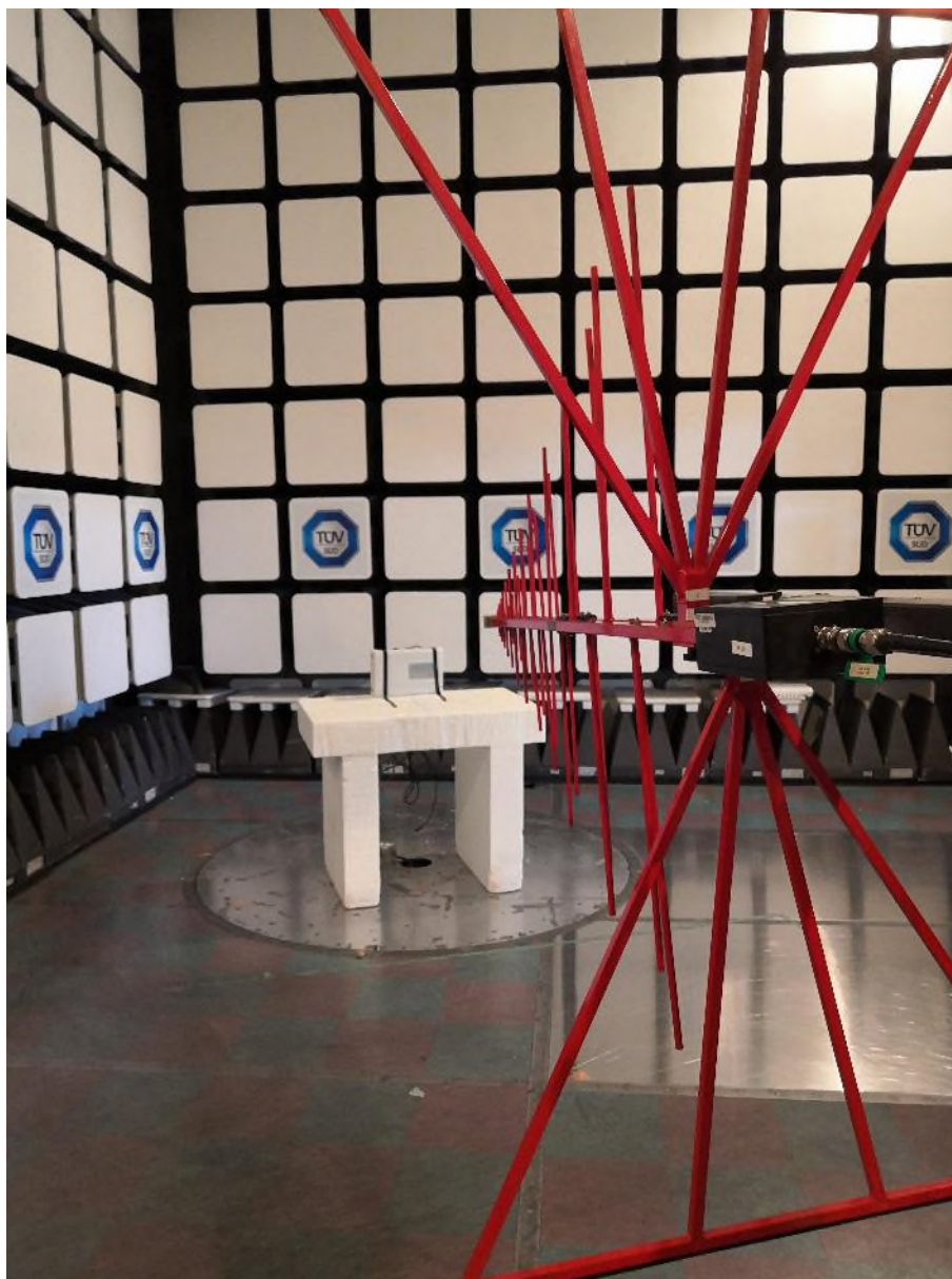
Figure 2 – Radiated Emissions Setup 30MHz to 1GHz
