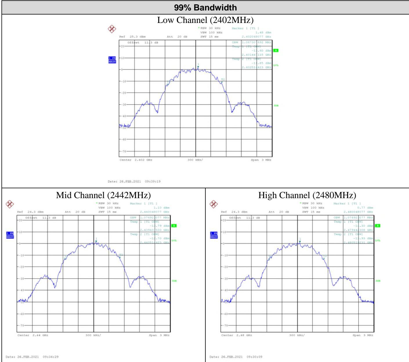
Note: See 'Appendix B – EUT & Test Setup Photos' for photos showing the test set-up.
