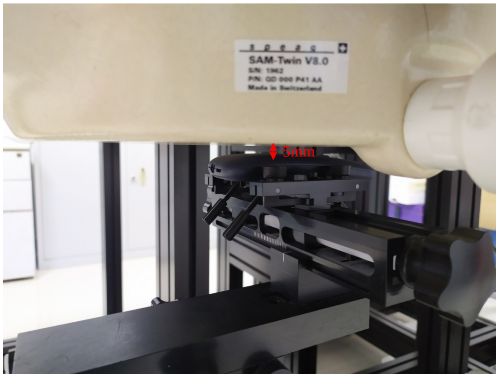
Body (Worn) Back Setup Photo (5mm)
