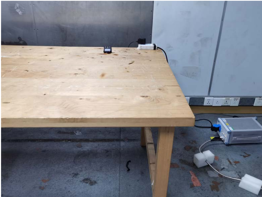
Photo of Power Line Conducted Emission Measurement
