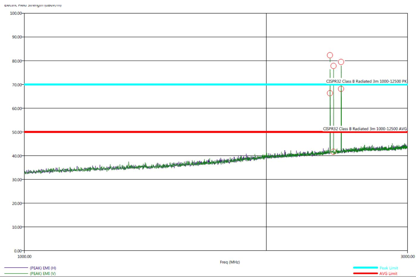
No emissions found from 1 GHz to 3 GHz. Emissions seen are from the pre-approved radio transmitter module that was tested separately.
