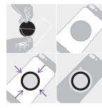
2. Align the magnetic sheet locator
