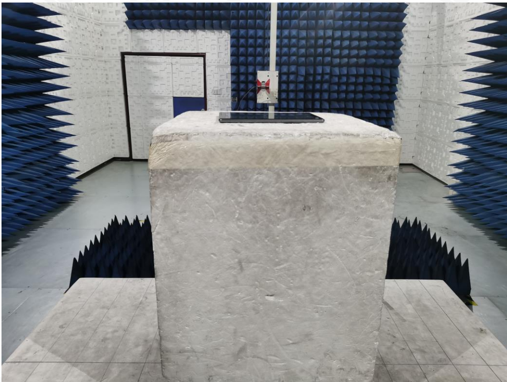
FCC RADIATED EMISSION TEST SETUP ABOVE 1GHZ
