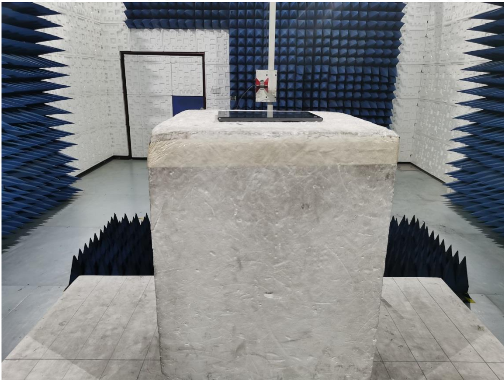
RADIATED EMISSION TEST SETUP ABOVE 1GHZ
