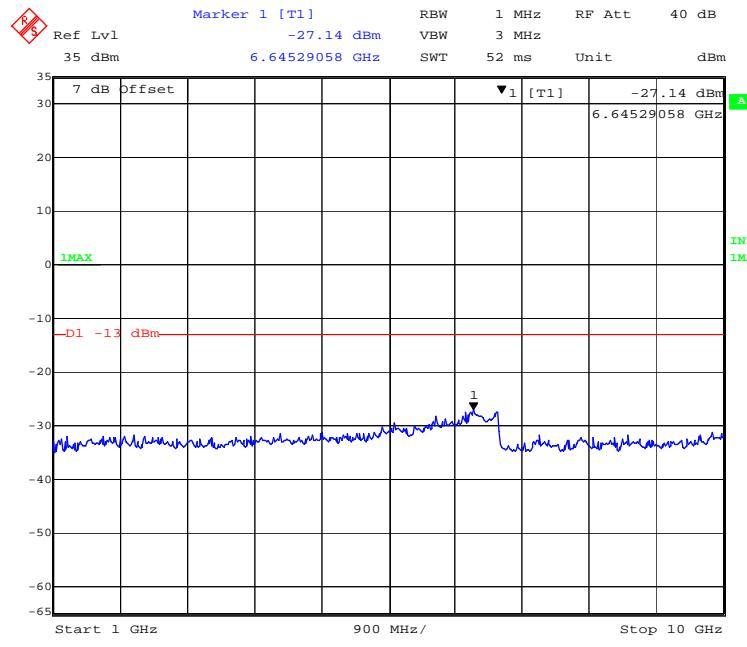
**Middle Channel****30 MHz – 1GHz(GPRS Mode)**
