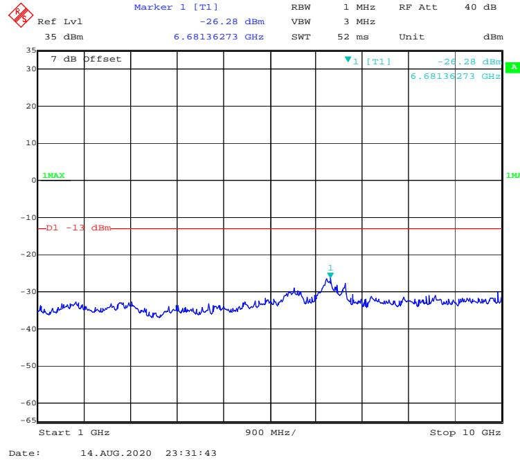
**High Channel****30 MHz – 1GHz WCDMA (HSUPA) Mode**
