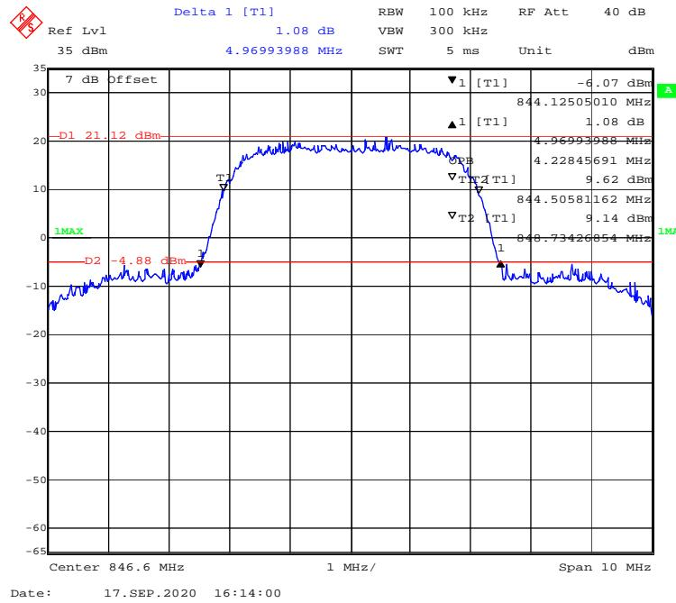
**PCS 1900Band****99% Occupied & 26 dB Emissions Bandwidth for GPRS (GMSK) Mode****Low channel**
