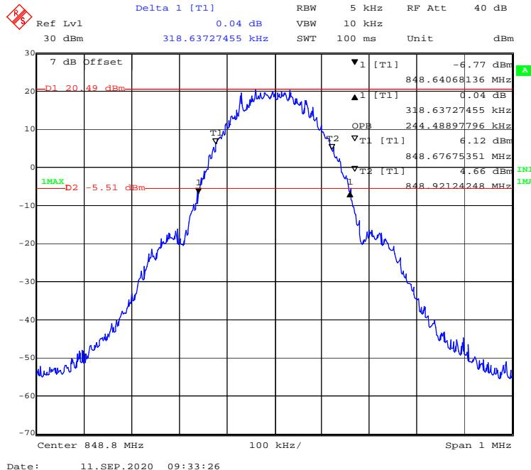
**WCDMA Band V****99% Occupied & 26 dB Emissions Bandwidth for WCDMA (Rel 99) Mode****Low Channel**
