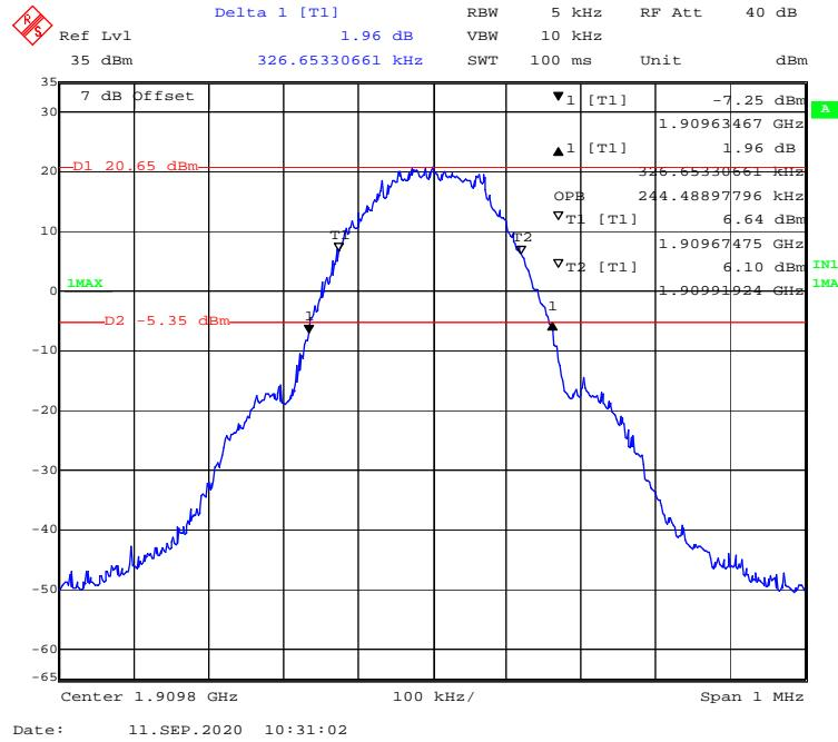
**WCDMA Band II****99% Occupied & 26 dB Emissions Bandwidth for WCDMA (Rel 99) Mode****Low Channel**
