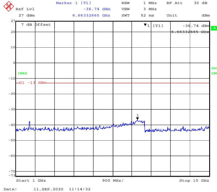
**Low Channel****30 MHz – 1GHz WCDMA (HSUPA) Mode**
