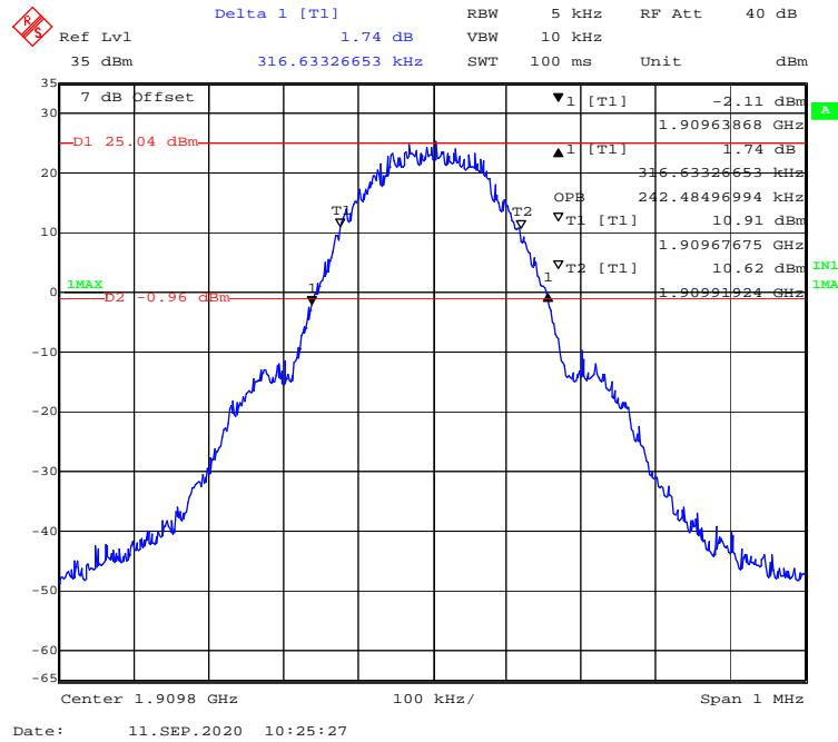
**99% Occupied & 26 dB Emissions Bandwidth for EGPRS (8PSK) Mode****Low Channel**
