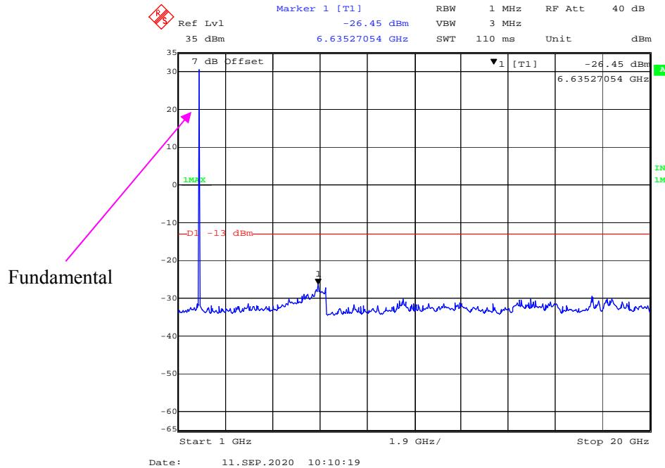
**Middle Channel****30 MHz – 1GHz(GPRS Mode)**
