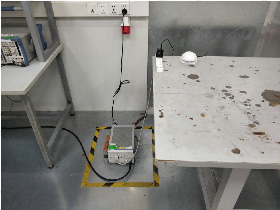
Photo of Conducted Emission Measurement
