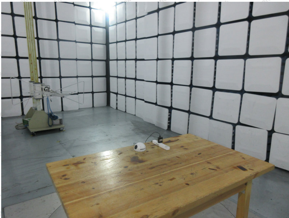
Photo of Radiation Emission Test
