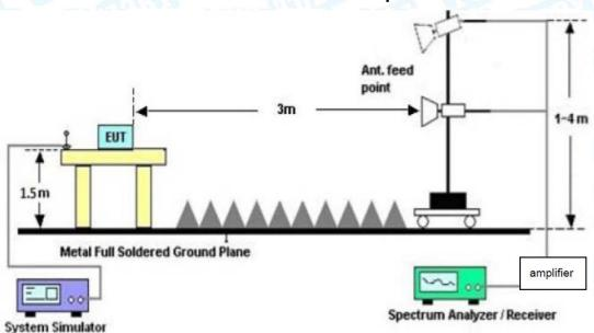
**Above 1GHz Test Setup**
