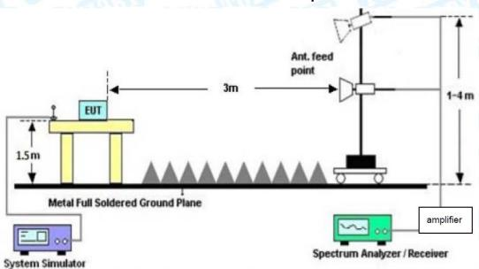
**Above 1GHz Test Setup**
