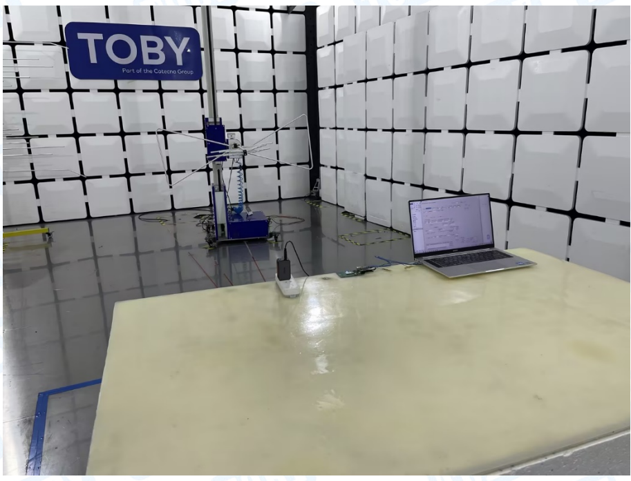
Photo of Setup for Radiated Emission (30MHz~1GHz)
