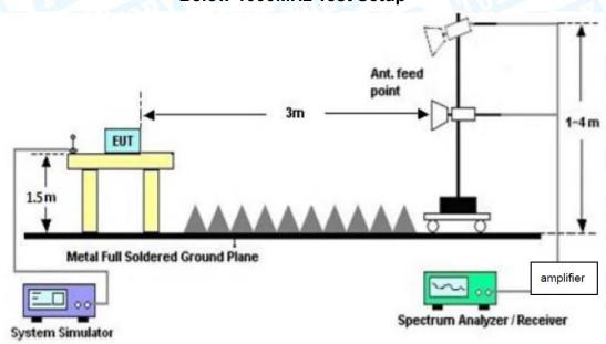
**Above 1GHz Test Setup**
