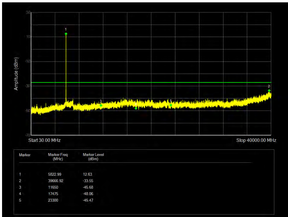
Tx. Spurious NVNT 802.11ac20 5825MHz Ant 2 Emission
