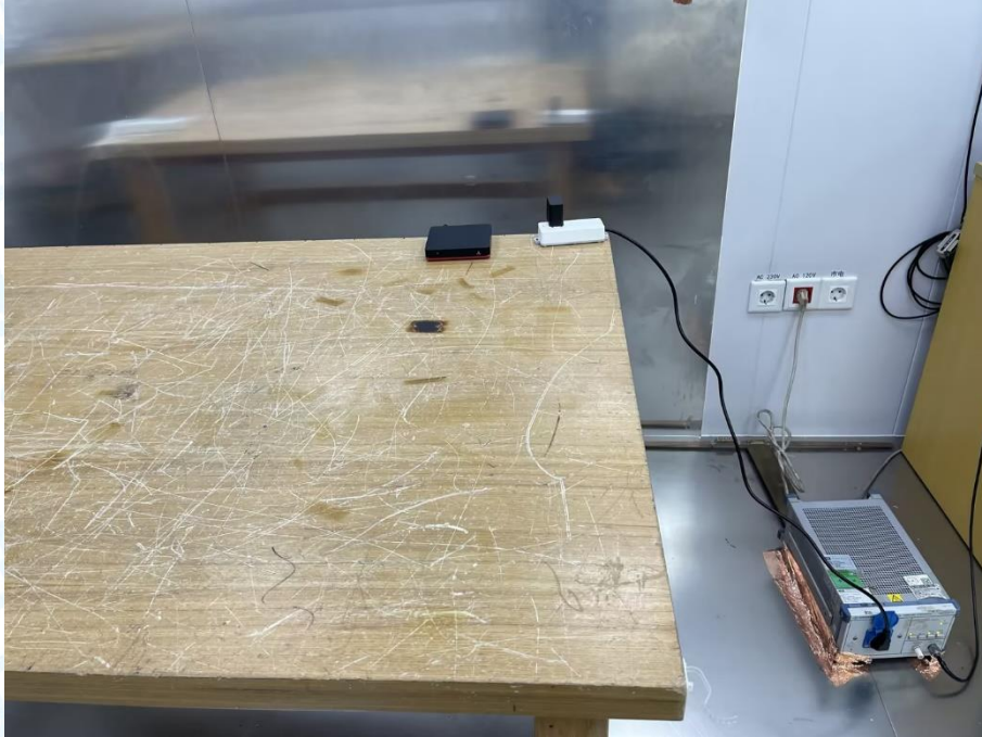
Photo of Setup for Radiated Emission (30MHz~1GHz)
