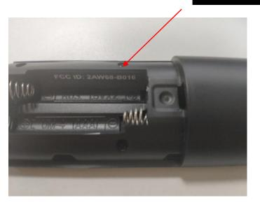
Label location: Battery Compartment Label size: 30mm\*6mm
