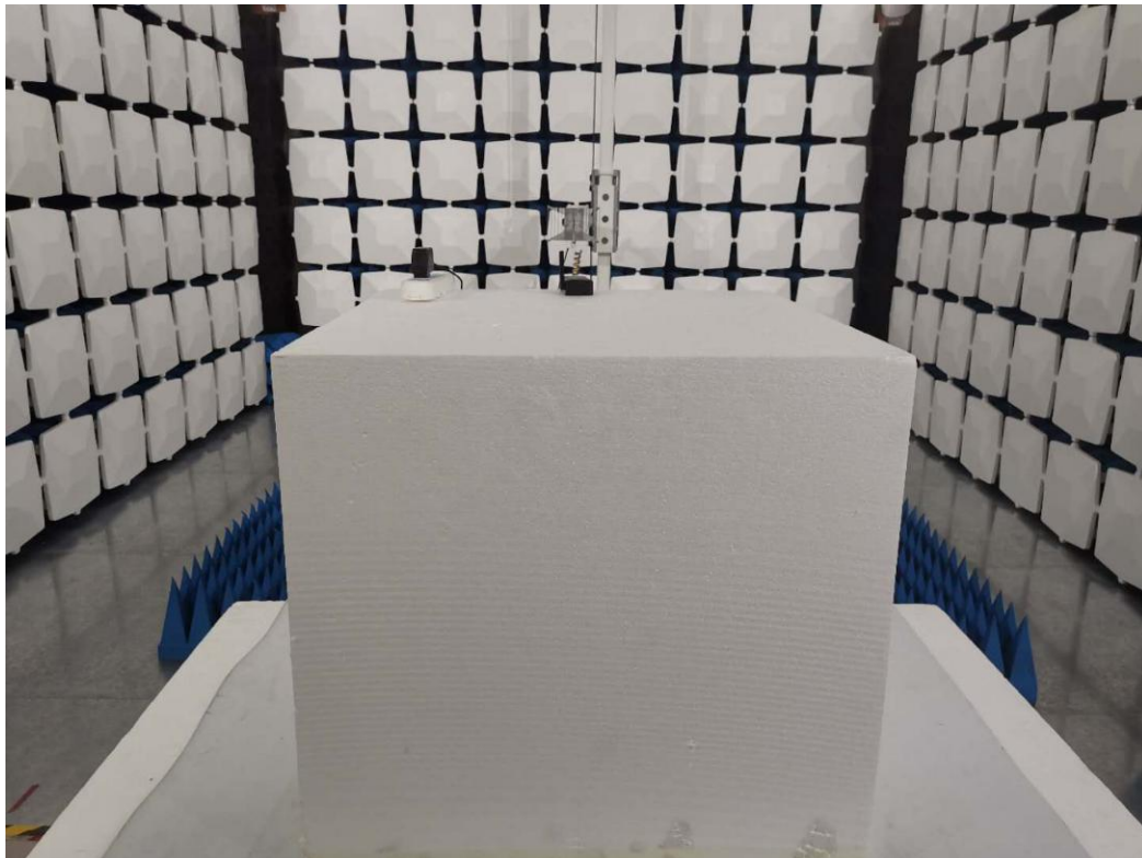
Above 1GHz for radiated emission test setup
