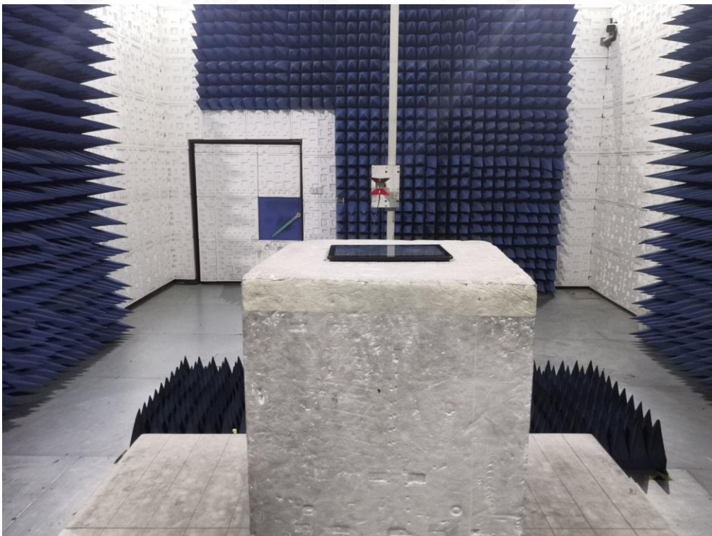
FCC RADIATED EMISSION TEST SETUP ABOVE 1GHZ
