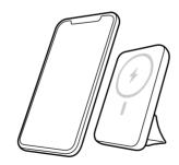
▲NOTE: Distance between your mobile device and the power bank should be no more than 6mm, most phone cases should not obstruct phone charging unless they are more than 6mm thick.
