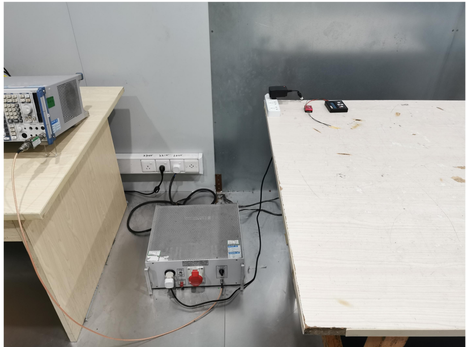
Conducted Emission Test Setup
