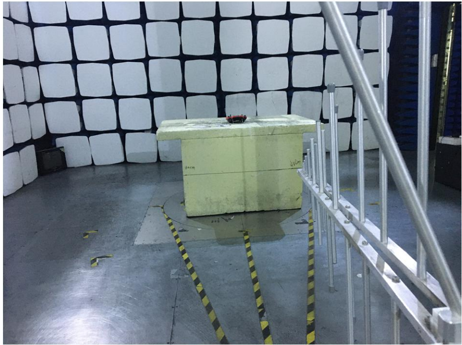
Radiation Emission Test Setup (30MHz to 1GHz)
