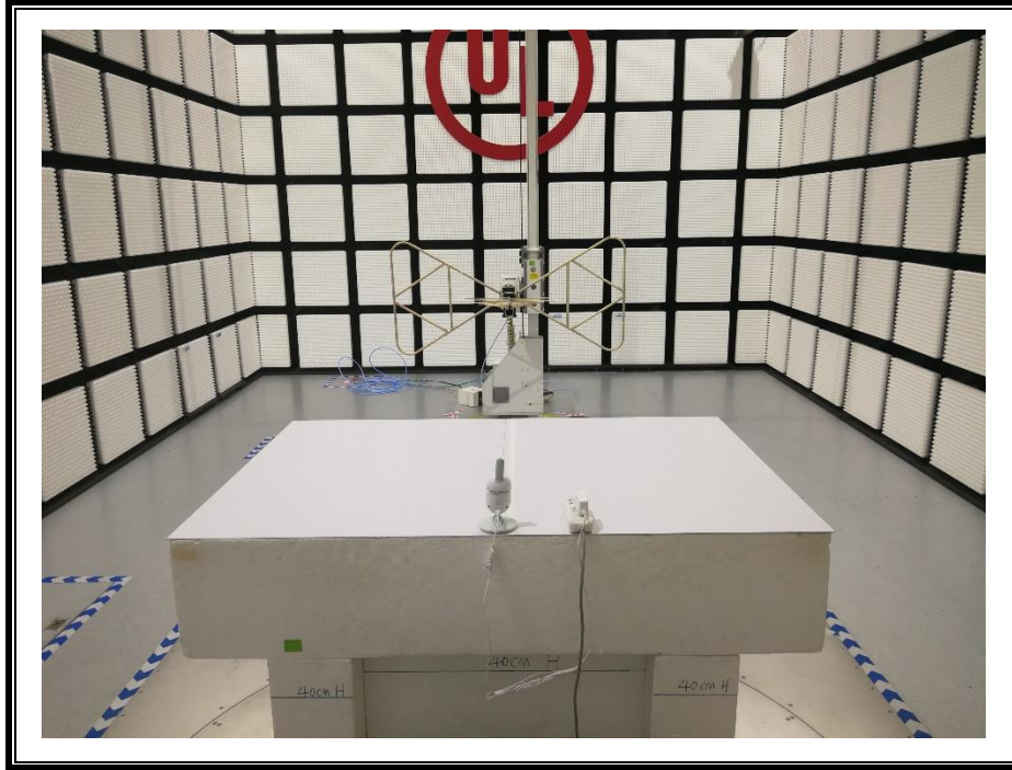
RADIATED RF MEASUREMENT SETUP (Below 30MHz) FOR PU
