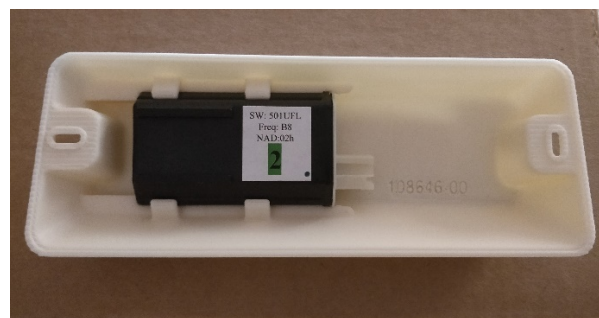
Figure 15: Sensor inserted in housing
