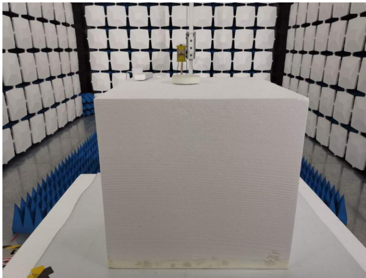
Above 1GHz for radiated emission test setup
