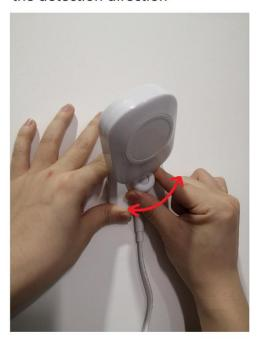
2. Shake the device to adjust the detection Angle
