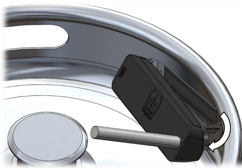
Step 4: Push removal tool fully into the second slot
