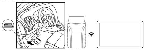
Plug the Wireless Diagnostics Module to vehicle's DLC port first, then connect the device via Wi-Fi.
