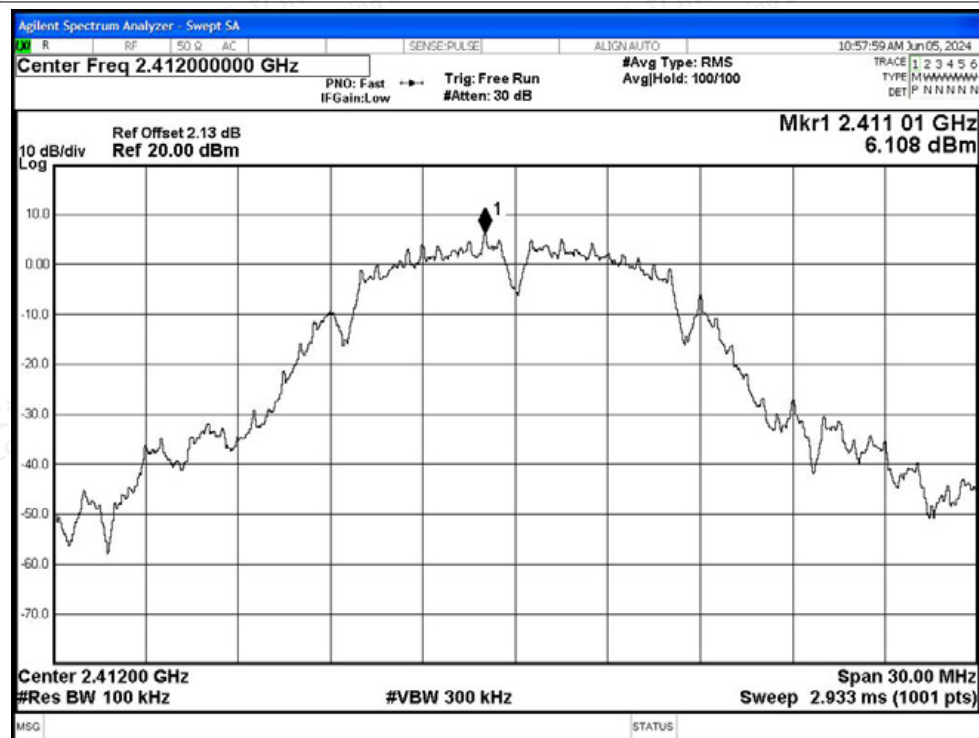
Band Edge NVNT b 2412MHz Ant1 Emission
