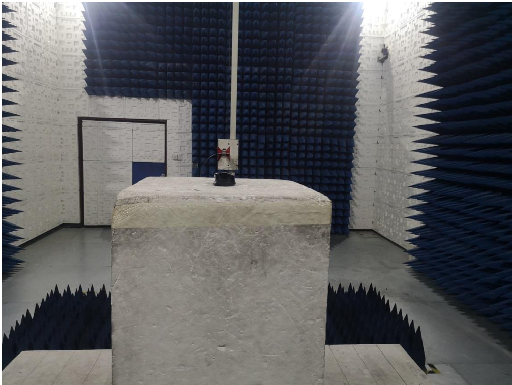
RADIATED EMISSION TEST SETUP ABOVE 1GHZ
