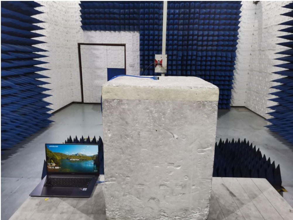
RADIATED EMISSION TEST SETUP ABOVE 1GHZ
