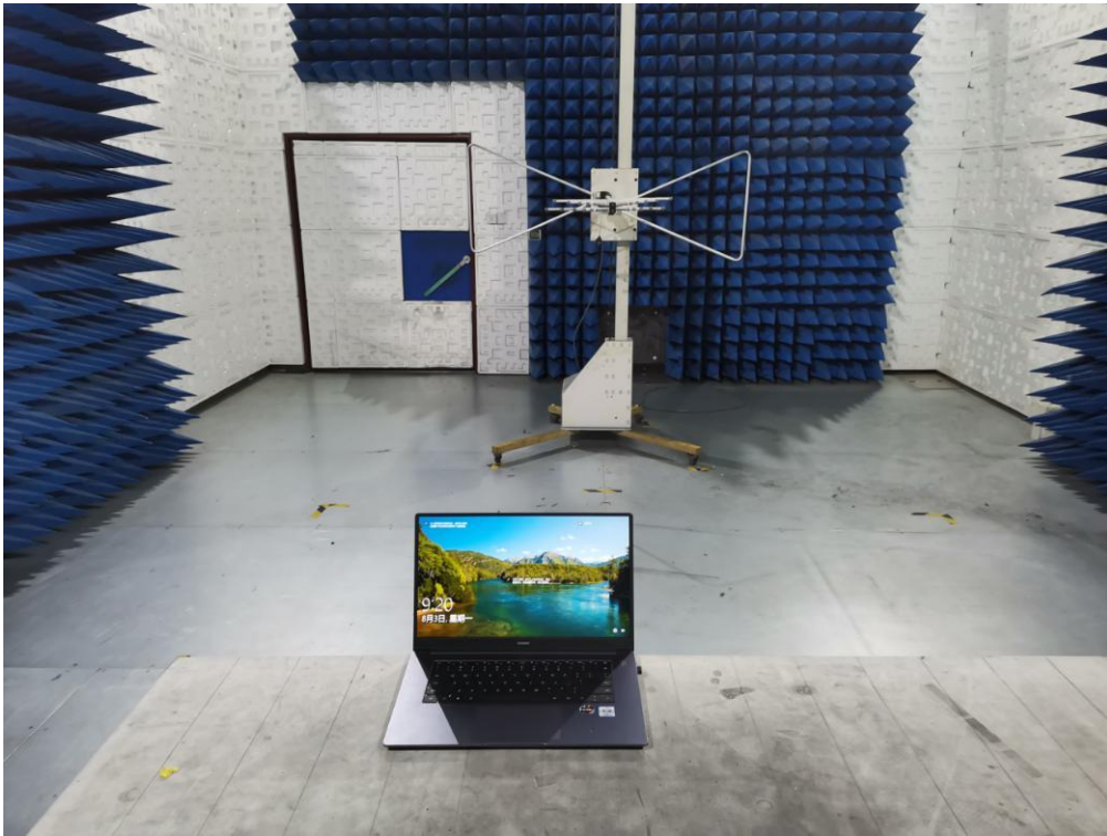
RADIATED EMISSION TEST SETUP ABOVE 1GHZ
