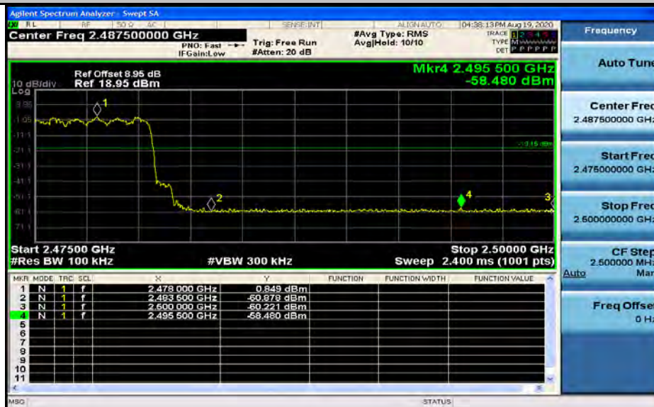
Band-edge for RF Conducted Emissions_2DH5_2480_Hopping Off
