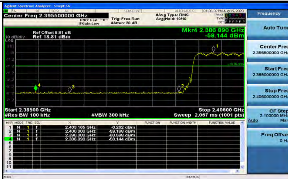
Band-edge for RF Conducted Emissions_2DH5_2402_Hopping Off
