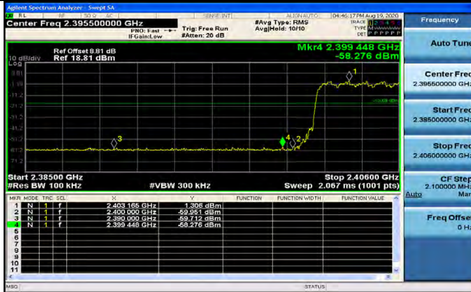
Band-edge for RF Conducted Emissions_3DH5_2402_Hopping Off
