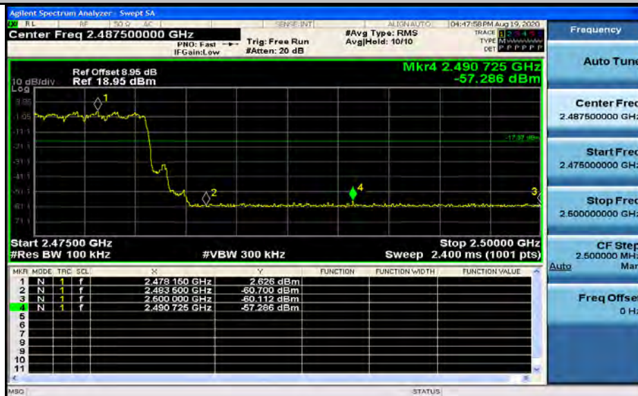
Band-edge for RF Conducted Emissions_3DH5_2480_Hopping Off
