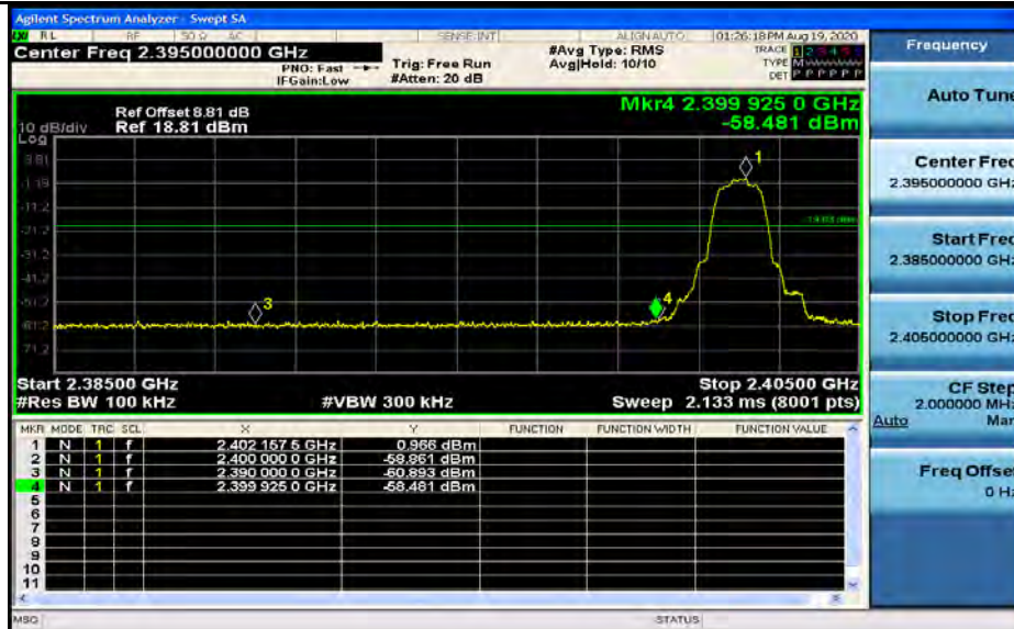
Band-edge for RF Conducted Emissions_2DH5_2480_Hopping On
