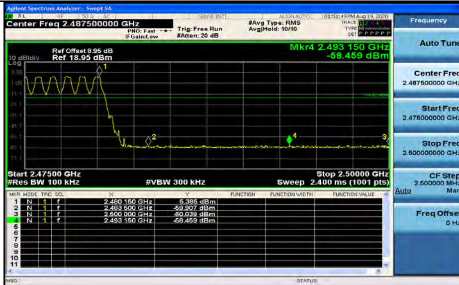
Band-edge for RF Conducted Emissions_DH5_2480_Hopping Off
