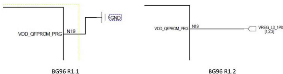
Figure 1: Schematic Designs of BG96 R1.1 and R1.2
