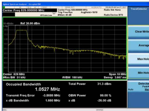
LTE Band 26 16QAM 10MHz CH-Middle
