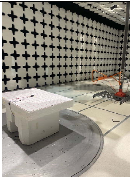
Radiated Emission Test below 1GHz Rear View
