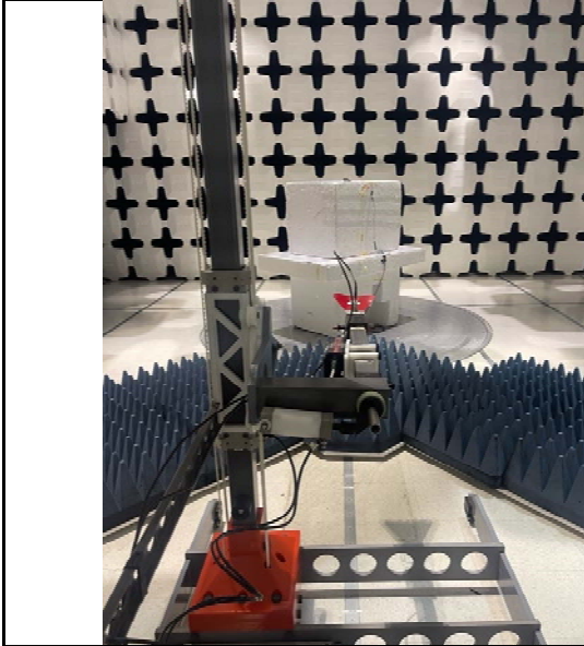
Radiated Emission Test Above 1GHz Front View
