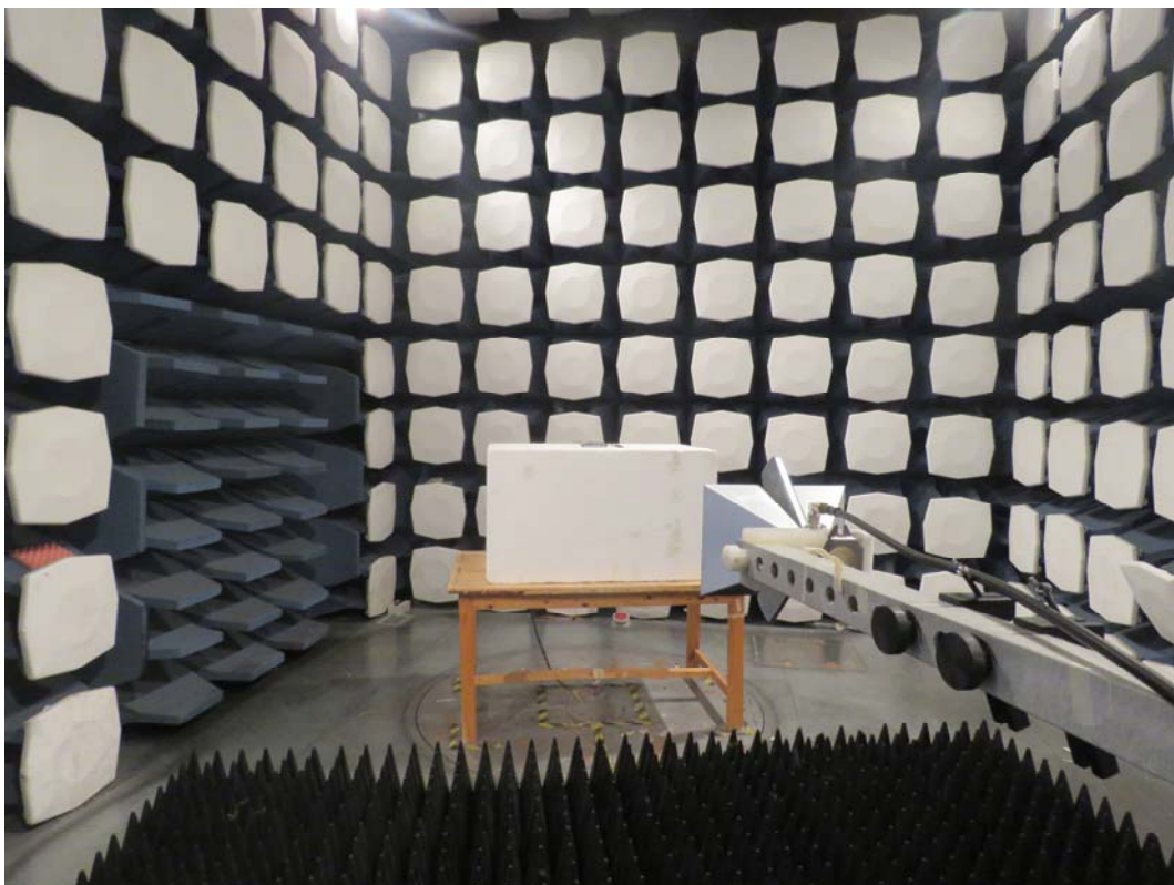
Picture 2 Radiated Spurious Emissions Test setup
