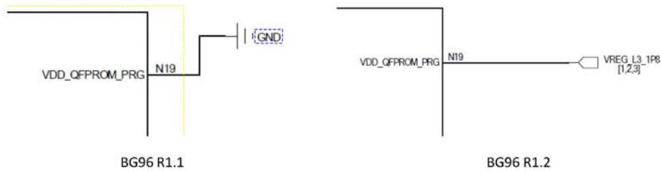
Figure 1: Schematic Designs of BG96 R1.1 and R1.2
