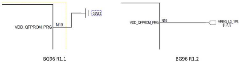
Figure 1: Schematic Designs of BG96 R1.1 and R1.2
