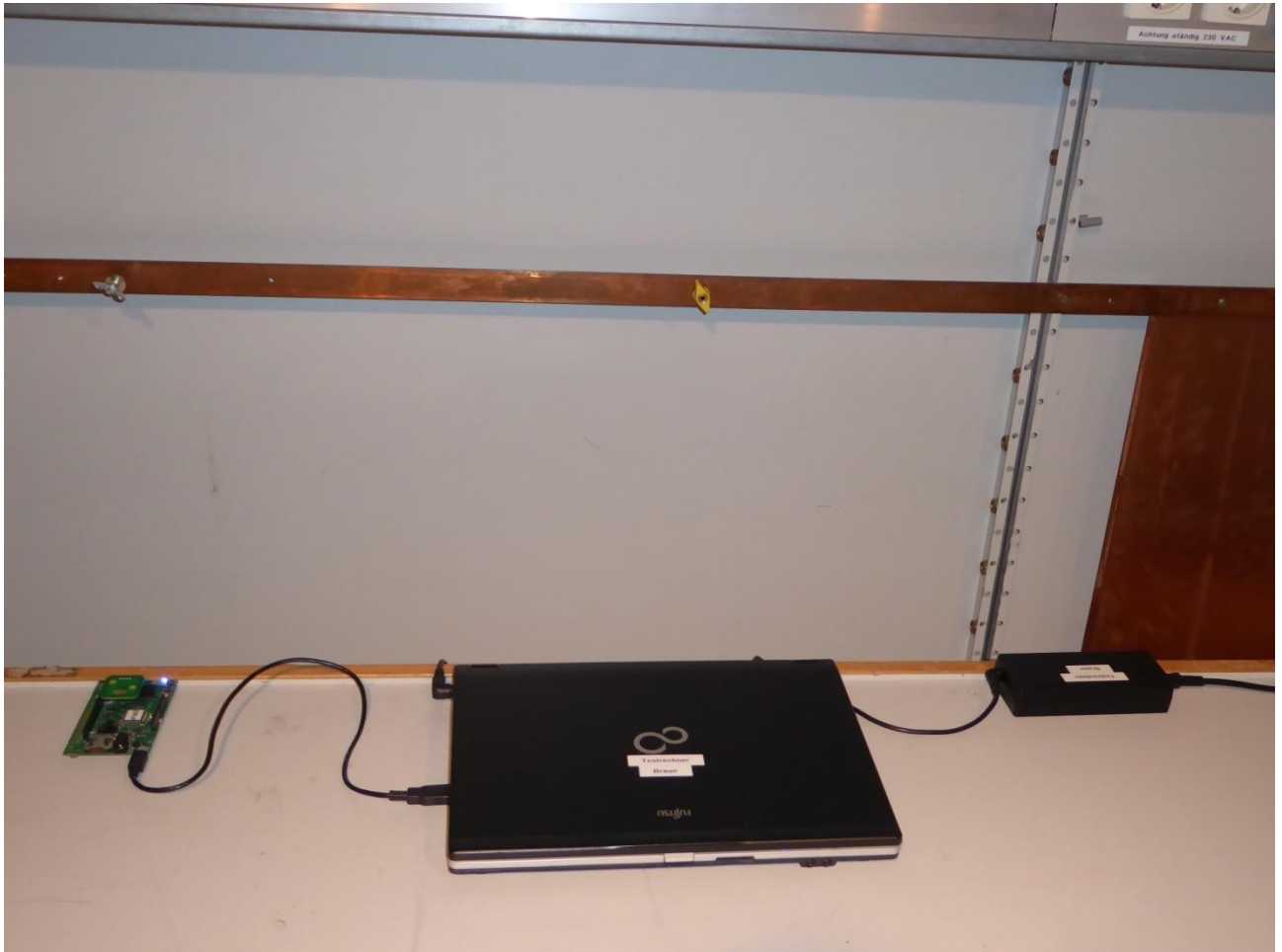
181323_SetMainsU1.JPG: Test setup mains conducted emissions; EVB-ANNA-B112U#117
