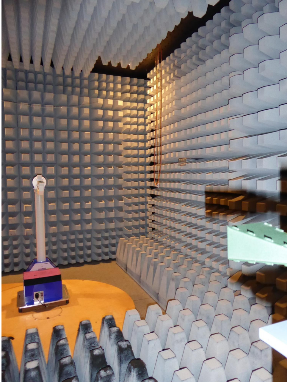
181323_SetRadC11.JPG: Test setup fully anechoic chamber; EVB-ANNA-B112C#143, 18 – 26.5 GHz
