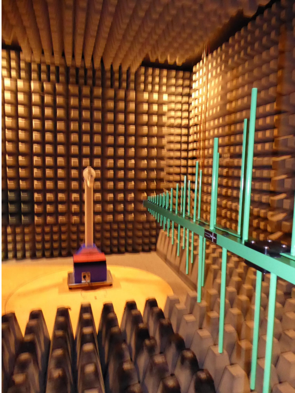
181323_SetRadU8.JPG: Test setup fully anechoic chamber; EVB-ANNA-B112U#117, 30 MHz – 1 GHz
