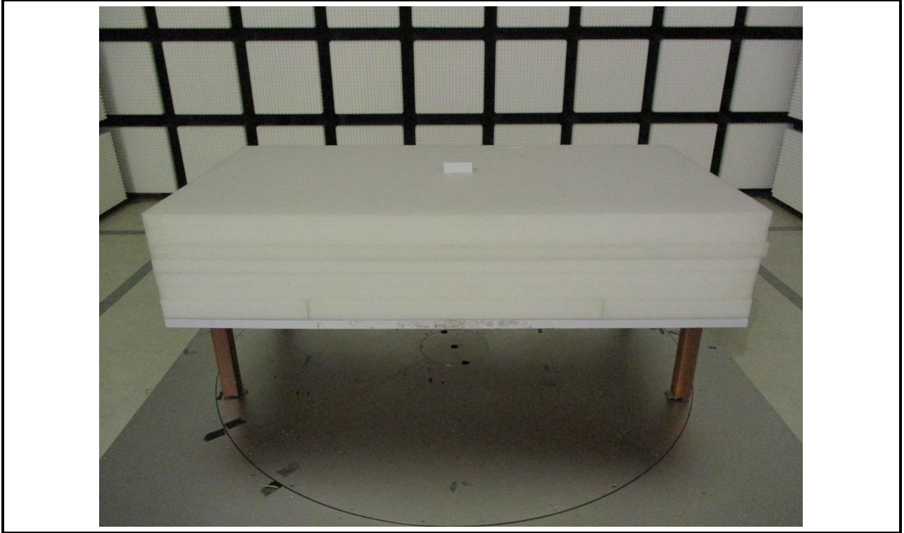
Radiated Emission Below 1GHz Test
